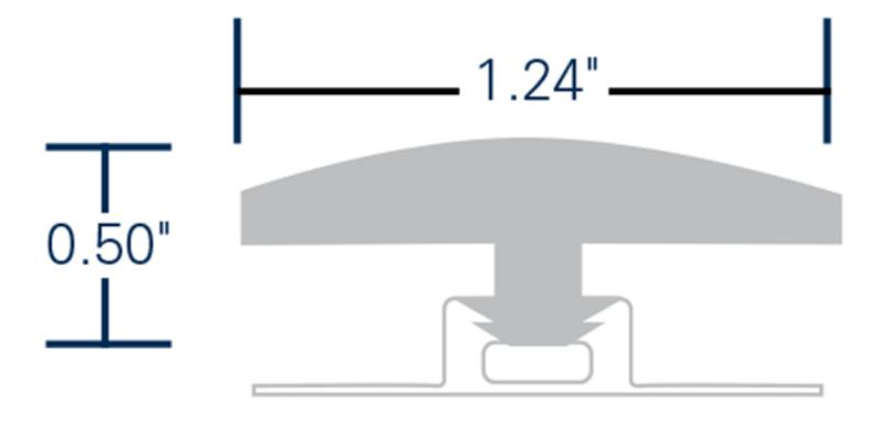
T-Mold and Overlap Reducer Installation
