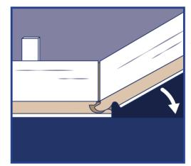
Step 2: Lock short end of flooring by inserting tongue into groove at an angle and drop in place. Continue to end of first row.
