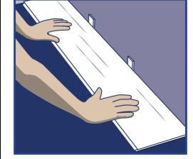
Step 1: Begin installation working from left to right. Insert spacers at ends and edges where flooring meet wall.
